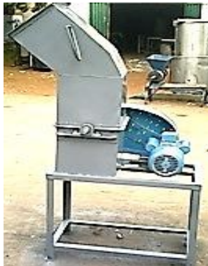
Figure 1: Thermoplastic Crushing Machine (a) CAD model (b) after construction
